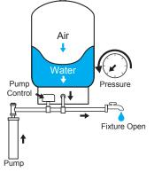
The larger the well tank, the greater the storage capacity and the less time the pump needs to run. This saves energy and extends pump life. Larger tank sizes also provide more consistent water pressure.
