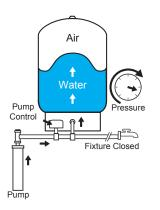
2. As water is used, it is drawn from the tank and the pressure inside the tank decreases. When the set pressure is reached, the pump starts and refills the tank.
