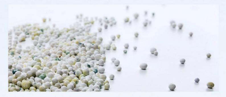
Far from the classical disinfection methods (chlorine, alcohol, bromide, ozone or UV), the QD ceramic catalysts have a discharged surface (a positive quantum field) that attracts electrons. Water simply has to pass over this media and the microorganisms (negatively charged) are instantly killed.
